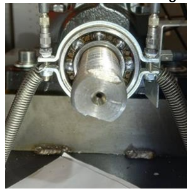
The outer race of the bearing admits rotational displacement.
